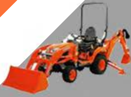
BX70 / BX25D 2013 Started offering drive over mower decks and moved the location of the brake pedal to the left side for more comfort. The BX70 also introduced the quick hitch.
