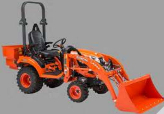
BX80 / BX23S 2017-Today Introduced the Swift-Tach loader, single piece hood redesign and offers a third function valve kit. The R14 tires were also introduced in 2021.
