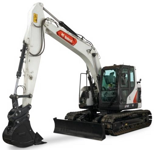
With its turbocharged 3.4 liter, non-DPF engine and class-leading hydraulics, the new Bobcat® E145 delivers a mighty combination of maneuverable size, high lifting capability and powerful breakout forces for prolific digging performance.
