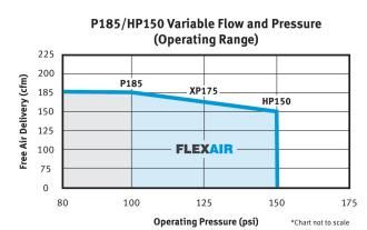
\*See Doosan FlexAir Variable Flow & Pressure chart for flow at given pressures
