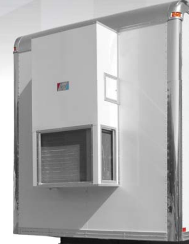
Bard A/C Mounted on Front Bunk (picture shows Bard unit covered with optional white aluminum)
